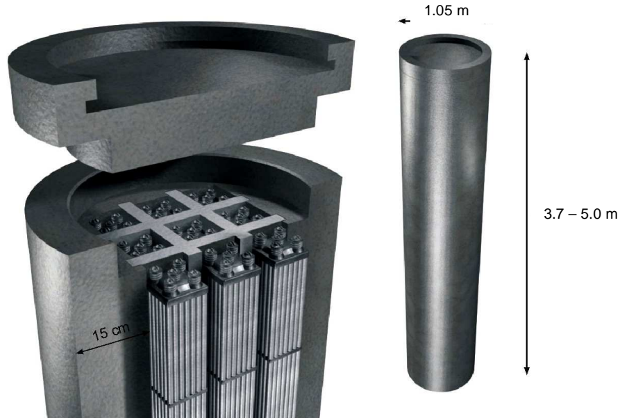
Figure 4: Preliminary design of the Swiss canister for the disposal of spent BWR fuel – possible reference design for SAPIERR disposal container
